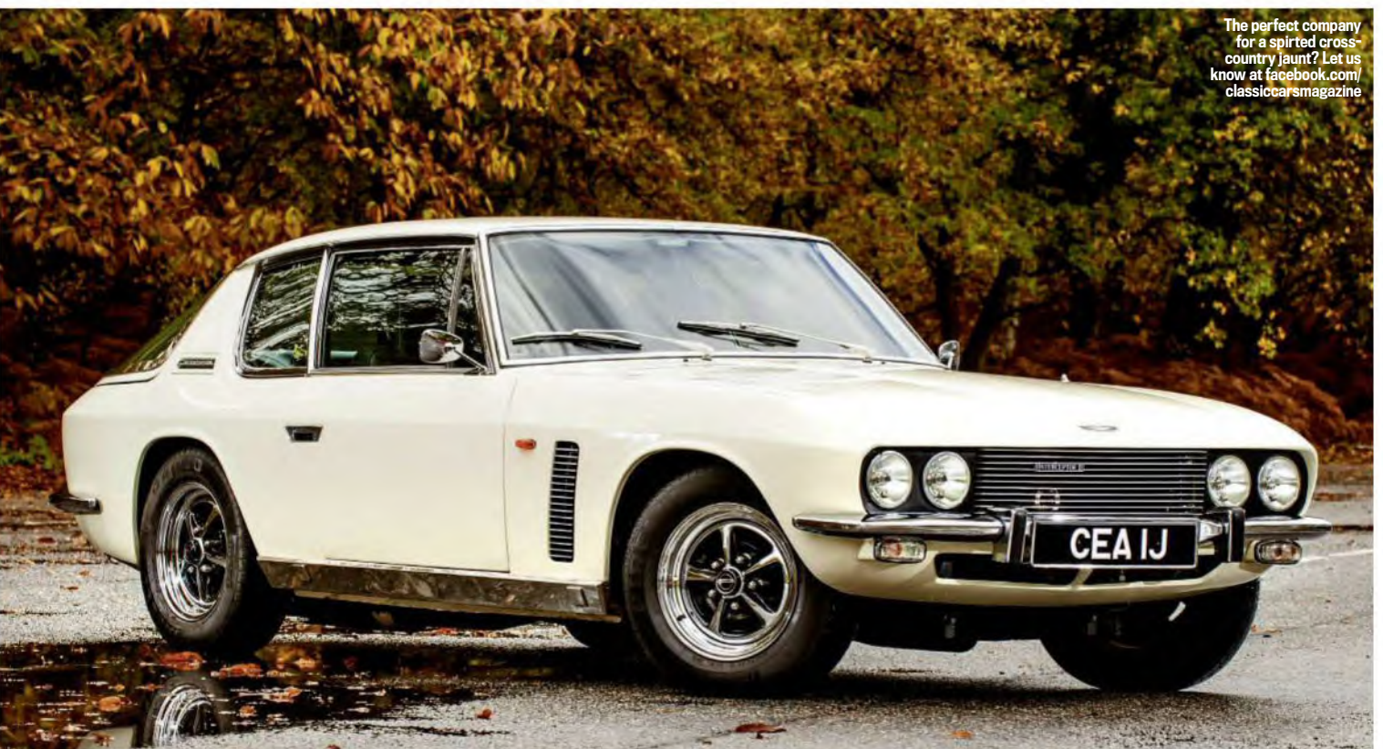
Interceptor II and III's handling was much improved by standard power-assisted steering and ball-jointed front suspension
