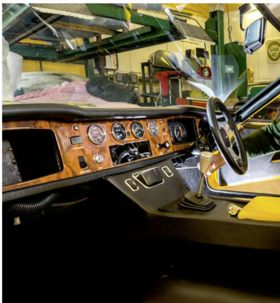
Dashboard fitting was a challenge thanks to 'a big lump of glassfibre in the way' – a legacy of poor previous repairs
