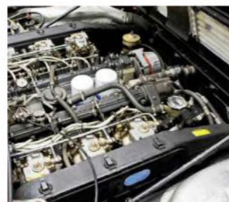
Vast 4.8-litre V12 delivers its 340bhp smoothly, with clean fluids and no leaks
