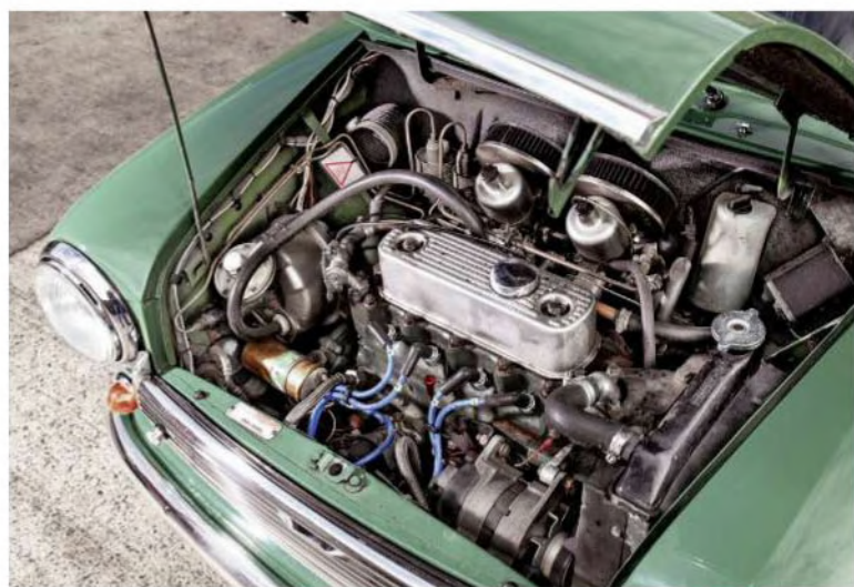
A-series looks standard but a host of modifications have boosted power to nearly 100bhp
